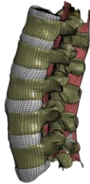
Figure 1 Hexahedral finite element model of a ligamentous lumbar spine based on quantitative computed tomography of a cadaveric spine.
