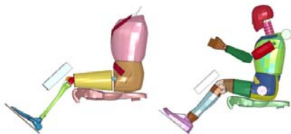
Figure 1. FE KTH (left) and FE Hybrid III (right) Models Positioned for Sled Test
