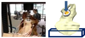
Figure 1: Loading condition for the experiment and FE analysis
